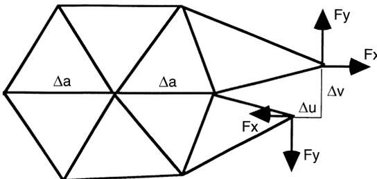
Fig. 5. Crack closure technique
