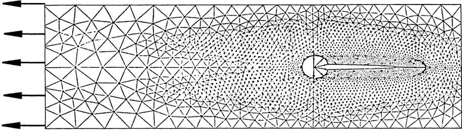
Fig. 4. Finite element mesh for a tension parallel to the grain and a central crack
