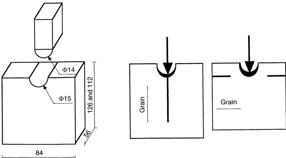
Fig. 3. ASTM specimens and degradation modes (Chaplain, 1996)
