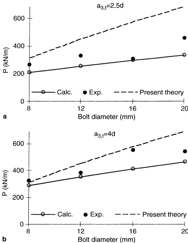
Fig. 9a, b. Tension parallel to the grain – Influence of bolt diameter – Short end-distances
