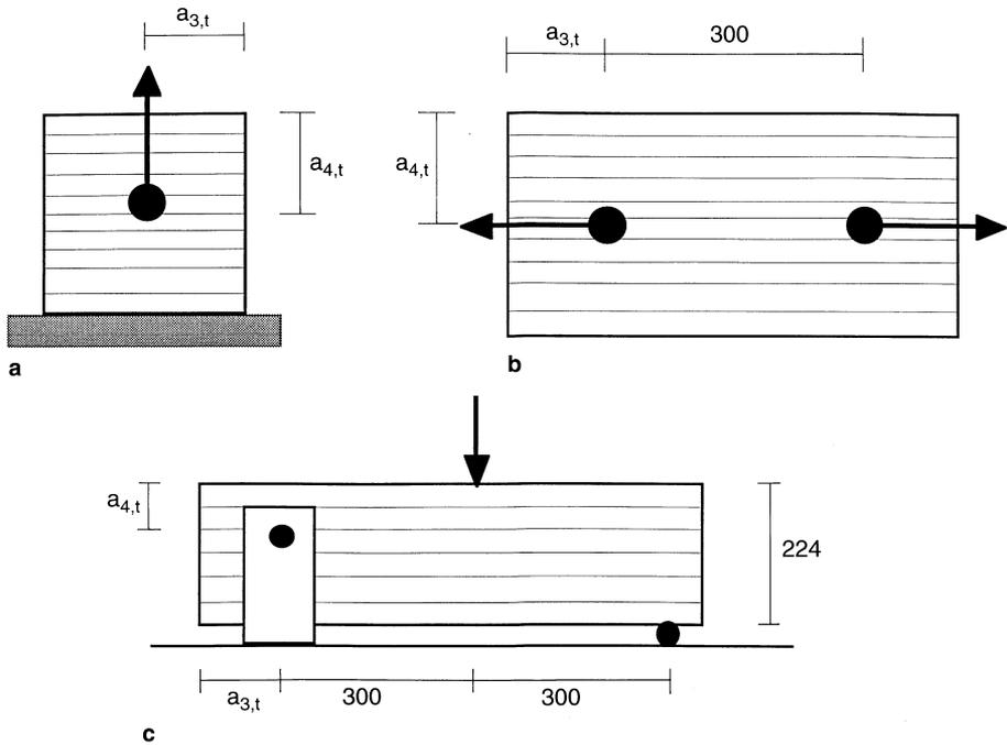
Fig. 1a-c. Specimens: a tension perpendicular to the grain, b tension parallel to the grain, c bending;  $a_{3,t}$  = end-distance,  $a_{4,t}$  = edge-distance
