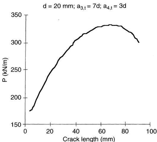
Fig. 6. Load versus crack length in tension perpendicular to the grain
