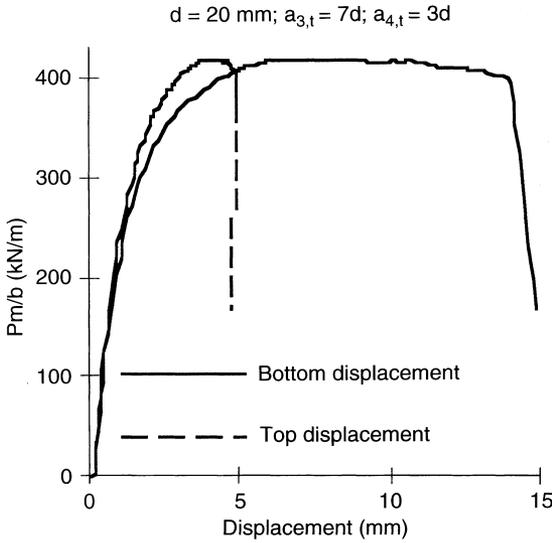
**Fig. 2.** Load-slip curves for a tension parallel to the grain
