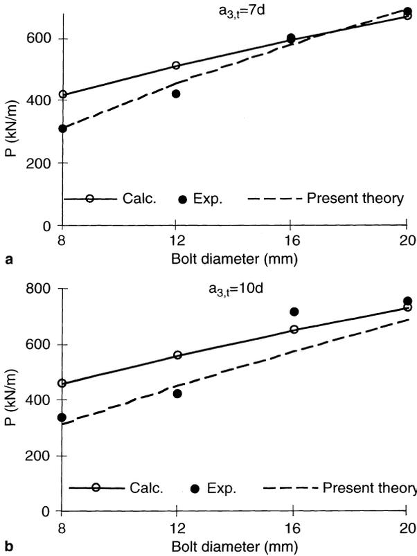
**Fig. 10a, b.** Tension parallel to the grain – Influence of bolt diameter – Conforming to the EC5 end-distances
