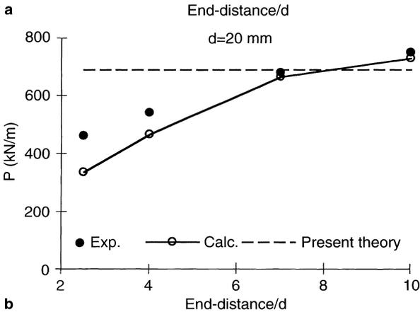
Fig. 11a, b. Tension parallel to the grain – Influence of the end-distance
