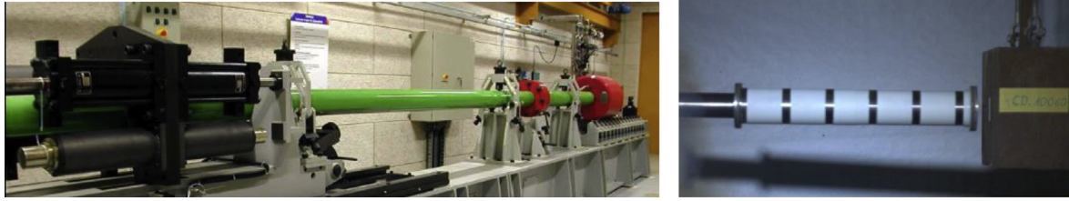
Fig. 2. Gas launcher, deformable projectile and ballistic pendulum device (just before impact) [7].
