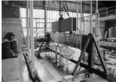
Fig. 2. Full-scale test of a beam
