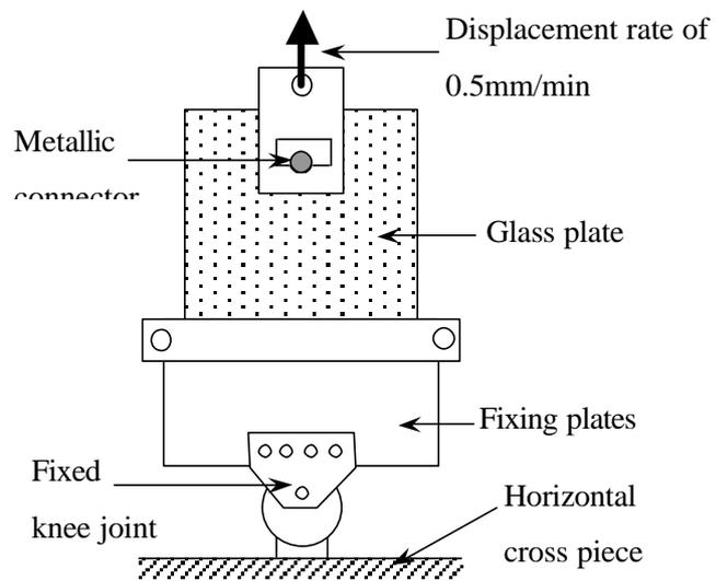
Fig. 8. Test set-up
