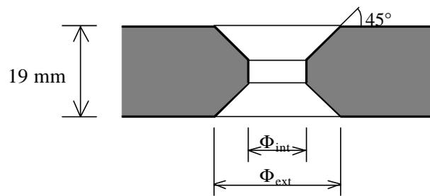
Fig. 4 .Chamfered hole
