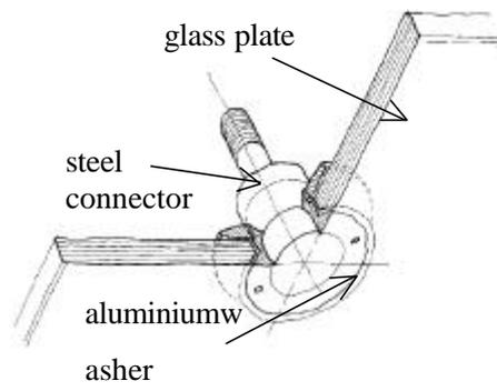
Fig. 3. Schematic view of the connection
