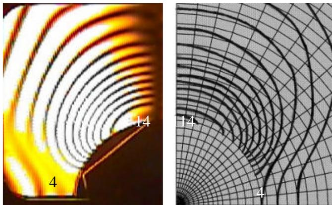
Fig. 9. Comparison between observed (left) and predicted (right) photoelastic fringes
