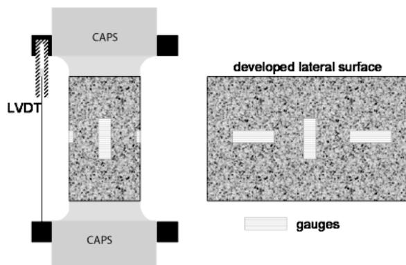
**Figure 2.** Scheme of strain measurement
