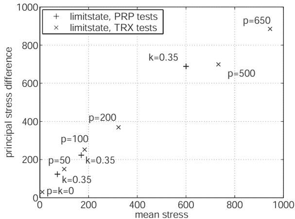
**Figure 7.** Limit states of concrete in the stress invariant space
