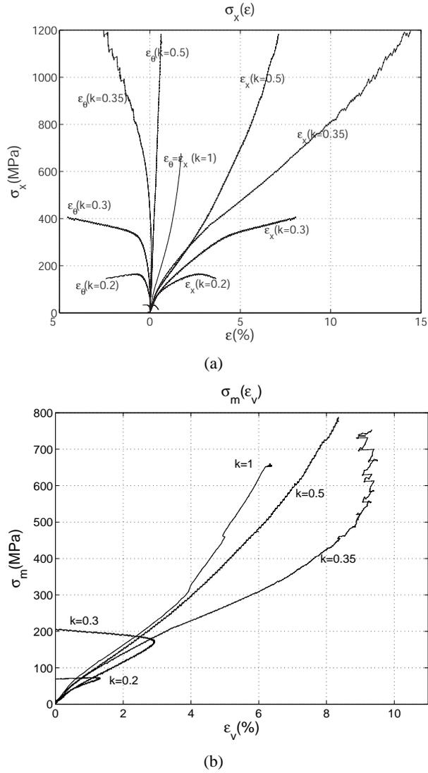
**Figure 6.** Proportional testing program : stress/strains curves (a) and volumetric behaviour (b).
