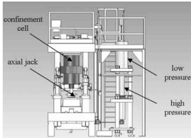
**Figure 1.** General scheme of the "GIGA" press
