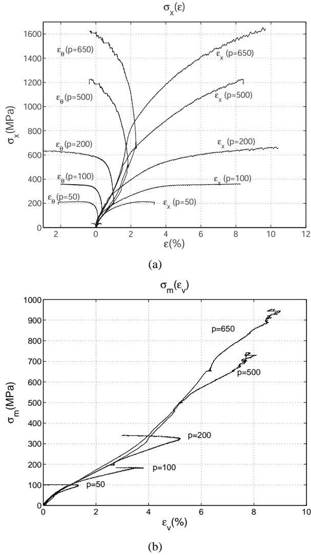
**Figure 5.** Triaxial testing program : stress/strains curves (a) and volumetric behaviour (b).
