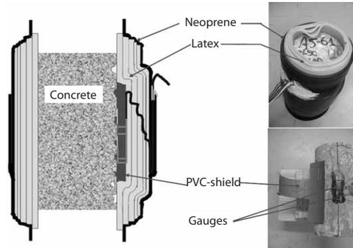
**Figure 3.** Vertical cross-section of a ready to test specimen
