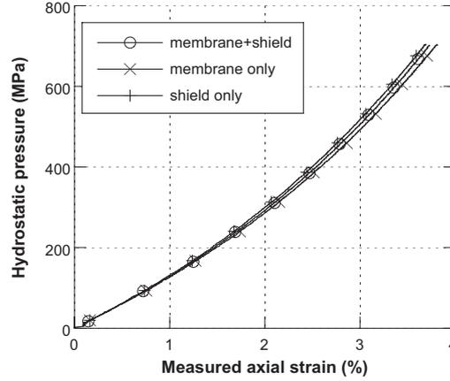
**Figure 4.** Influence of the PVC-shield and the membrane on measurement
