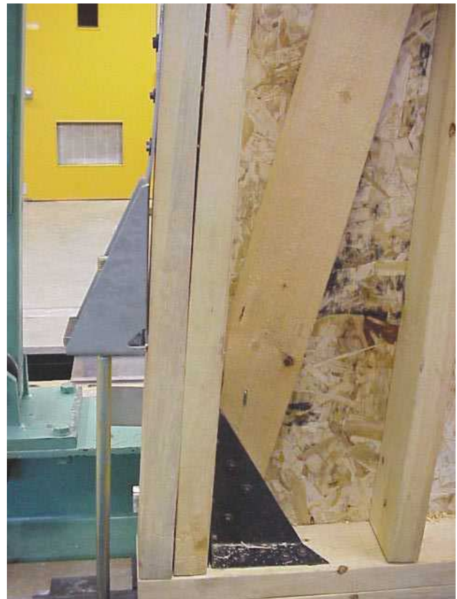
Fig. 8. Hold-down device and bracing system of wall 2.
