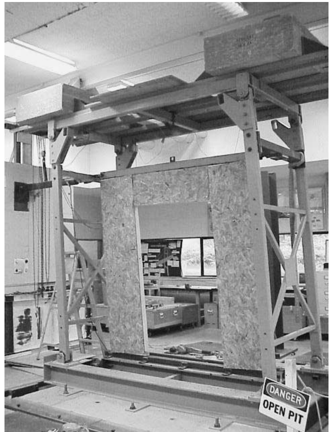
Fig. 6. Example of a shear wall test.
