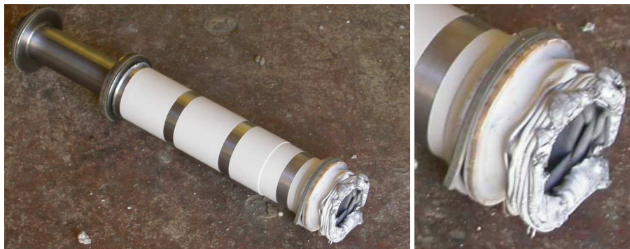
Figure 5. Deformation of the missile after perforation (test n°2, V_0 = 70.2 m/s)
