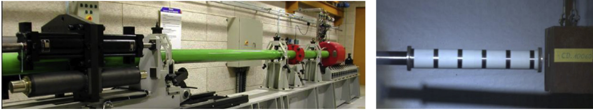
Fig. 2. Gas launcher, deformable projectile and ballistic pendulum device (just before impact) [7].
