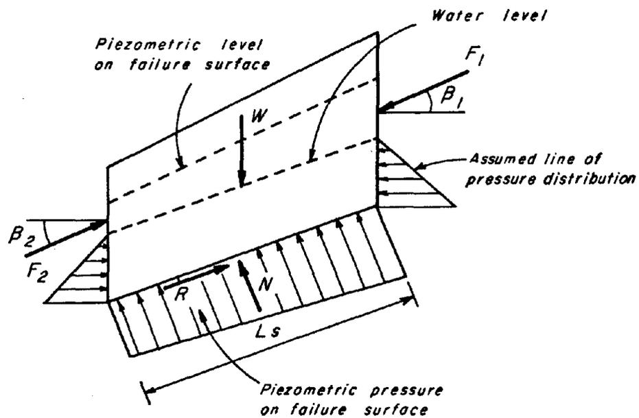
$W$  = total weight of soil and water above the failure surface
