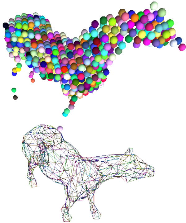
Figure 4.3: Imported GTS surface (horse) used as packing predicate (top) and surface constructed from facets (bottom). See http://www.youtube.com/watch?v=PZVruIIUX1A for movie of this simulation.
