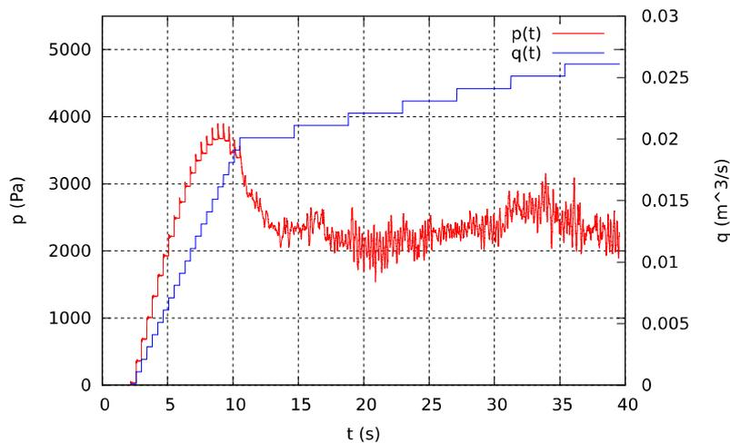
Figure 2. Evolution of the pressure in the time when the flow rate is increased from  $0.0001 \text{ m}^3/\text{s}$ , till  $0.0261 \text{ m}^3/\text{s}$  with increments of  $0.001 \text{ m}^3/\text{s}$  (27 steps)
