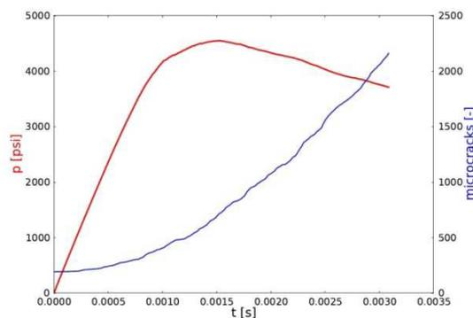
Figure 3 – Crack and pressure history (time in seconds).
