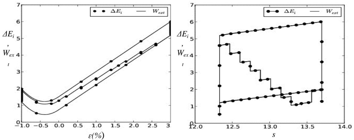
Figure 6. The plots of the external work and the total internal energy stored in the system as function of strain and suction
