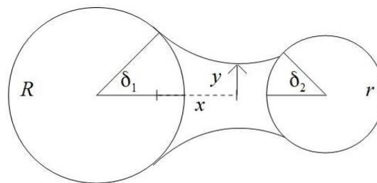
Figure 1. **Illustration of a liquid bridge between 2 spherical particles.**
