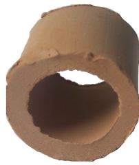
Figure 1: Cylindrical shell – a brittle constituent of highly porous granular material.
